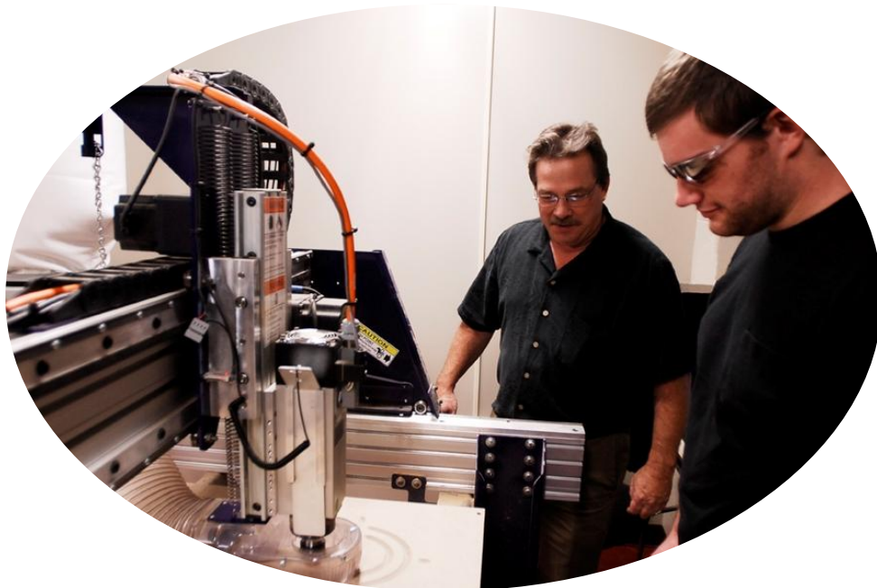
Instructor demonstrates the use of the FAB Lab Shop Bot to make a sign
